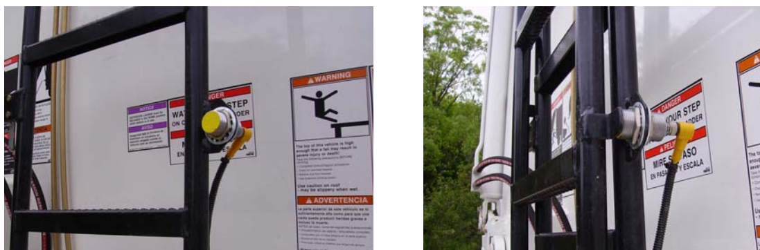
Figure 2-4 Extension Ladder Proximity Switch with ladder deployed (left) and in stored position (right).
