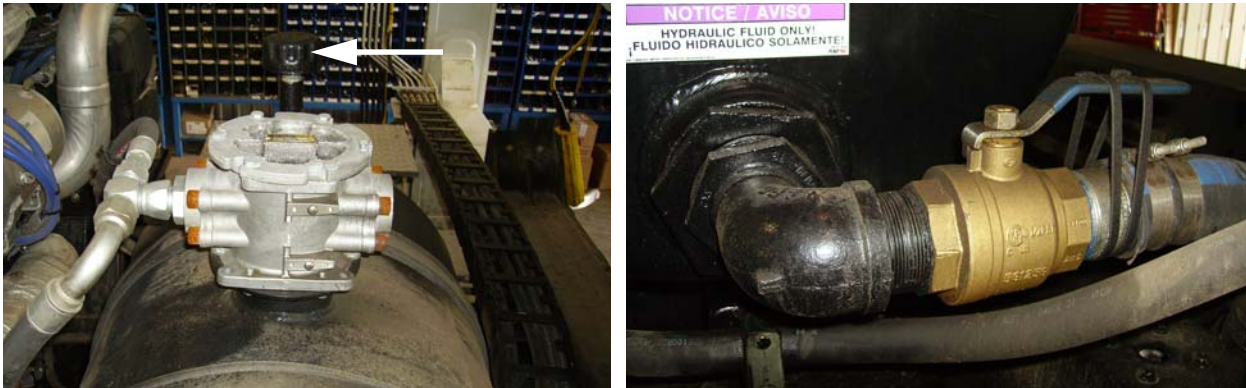
Figure 3-3 Breather cap, left / ball valve, right
