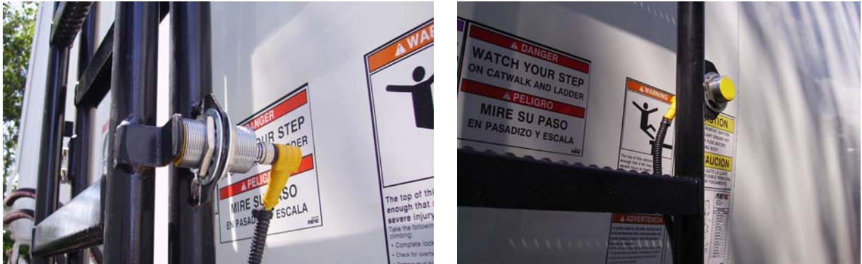
Figure 3-21 Access ladder proximity switch, ladder in “home” position, left; ladder in deployed position, right
