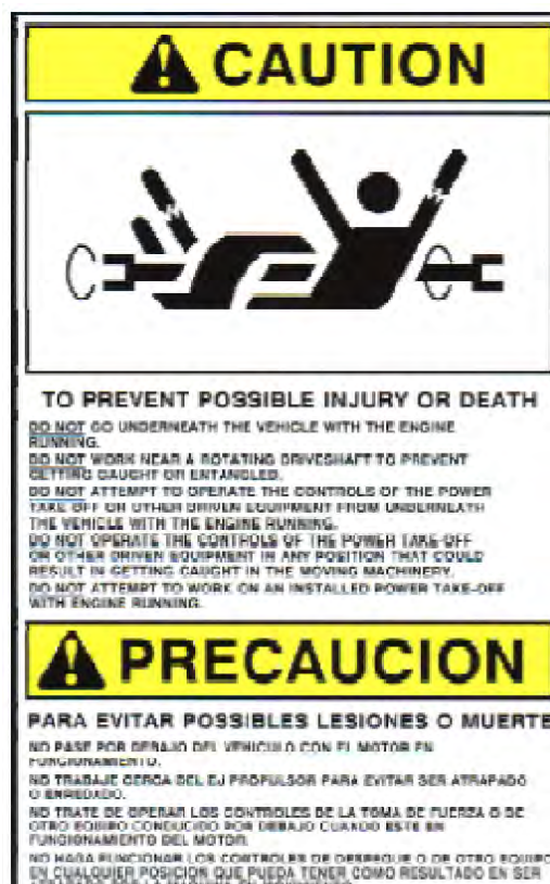
P/N 0605-859 CAUTION PTO HAZARD Located on both side of vehicle, on the frame rail.
