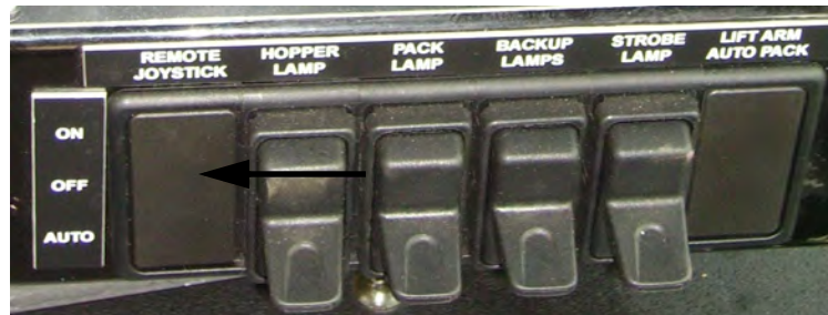
Figure 3-11 Location of the remote joystick control
