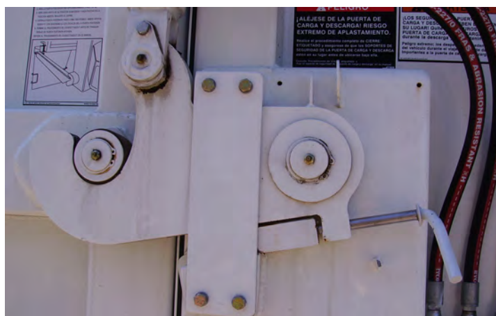
Figure 2-11 Tailgate safety locks in removed position
