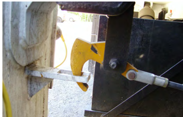
Figure 2-27 Lift lock in engaged position
