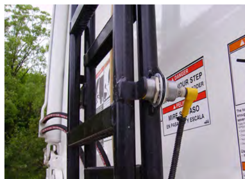
Figure 2-4 Extension Ladder Proximity Switch with ladder deployed (left) and in stored position (right).
