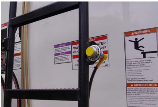
Figure 2-4 Extension Ladder Proximity Switch with ladder deployed (left) and in stored position (right)
