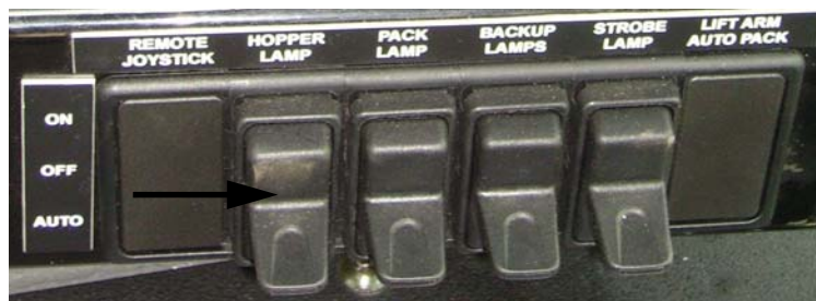
Figure 3-12 Hopper lamp switch
