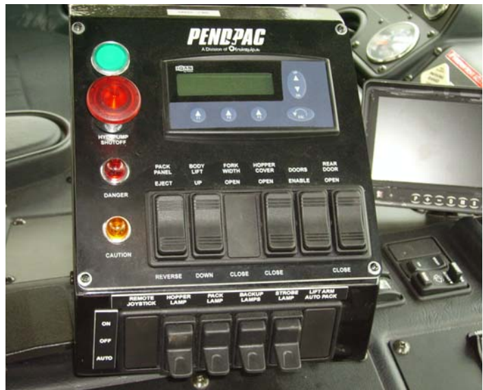
Figure 3-1 In-cab control console
