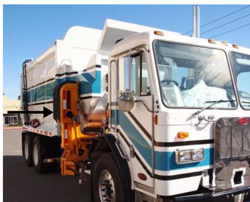
Figure 2-16 Slide retracted and in "HOME" position
