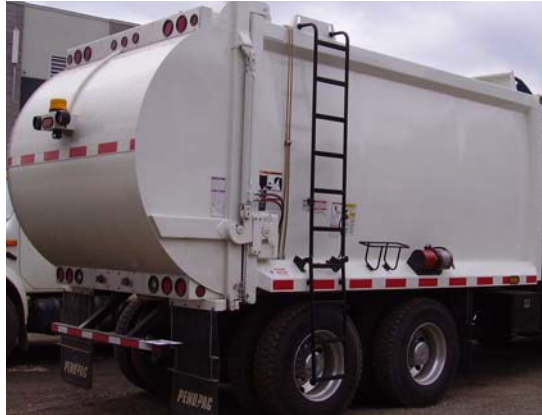
Figure 2-13 Access ladder in deployed position
