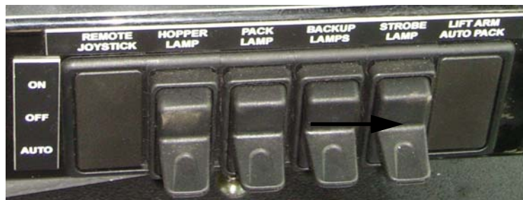
Figure 3-15 Strobe lamp switch
