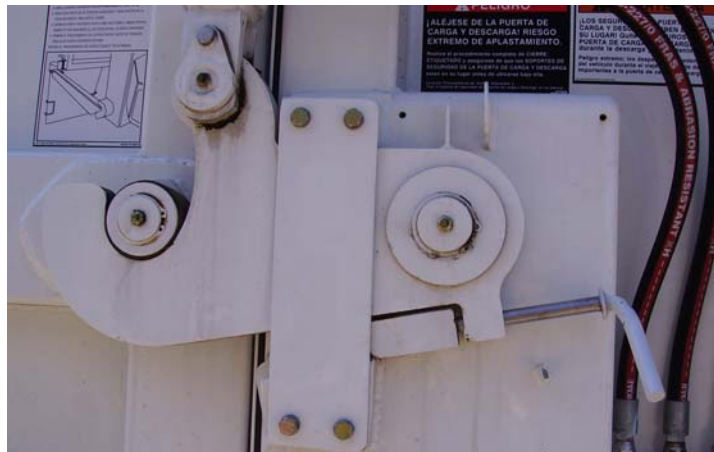
Figure 2-11 Tailgate safety locks in removed position
