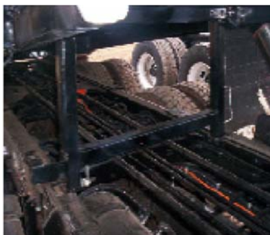
Figure 2-23 Hoist safety prop in engaged position
