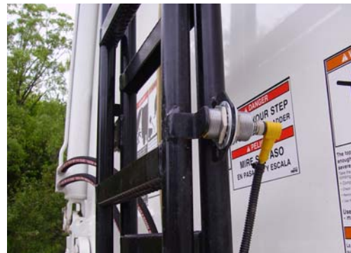
Figure 2-4 Extension Ladder Proximity Switch with ladder deployed (left) and in stored position (right)
