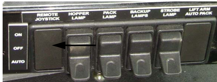
Figure 3-11 Location of the remote joystick control
