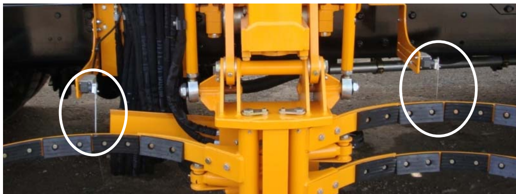
Figure 2-15 Arm limit switches
