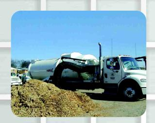
The Predator combines the strength of an Impac with a collection system for leafs and light debris. This year-round multipurpose trash and refuse vehicle is unmatched in its versatility. The super-hardened AB (Abrasive Resistant) steel mulching blades chop small branches, leaves, and grass cuttings (wet or dry) into tiny bits allowing for greater load compaction.
