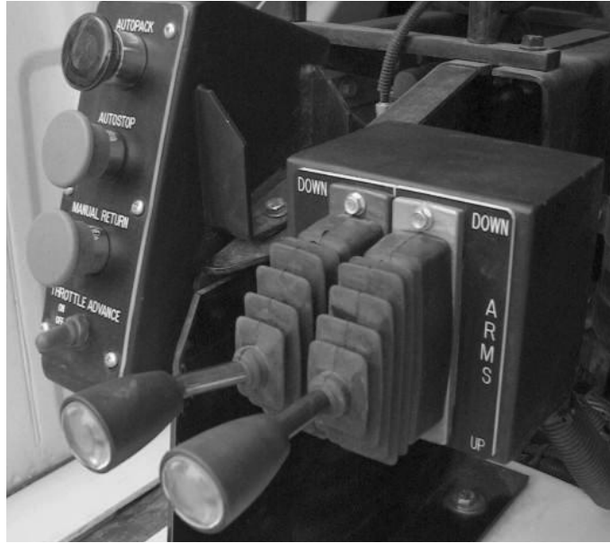
Figure 3-28 Outside controls (mounted behind cab)
