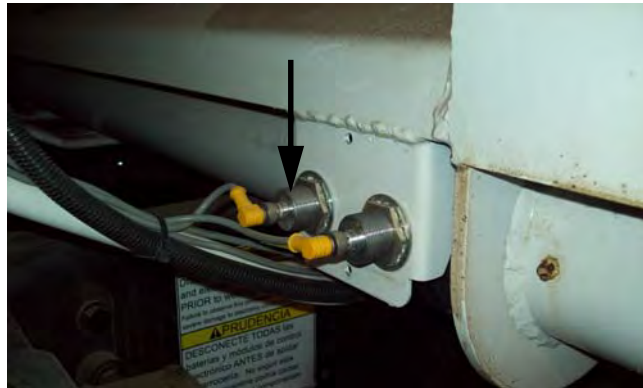
Figure 3-20 Arm partially raised proximity switch
