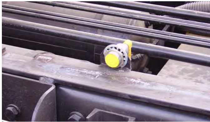
Figure 3-24 Body raised proximity switch
