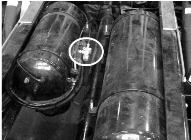
Figure 3-25 Chassis air tanks with 90 psi check valve highlighted
