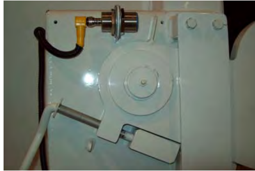
Figure 3-18 Tailgate ajar proximity switch (protective cover removed)
