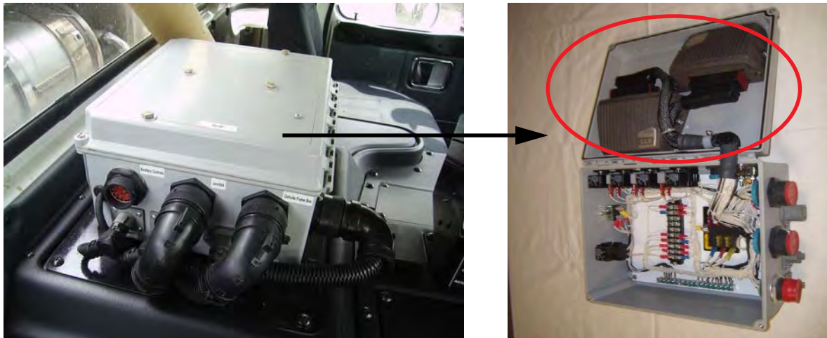
Figure 3-4 In-cab extension modules (100 and 200 series)
