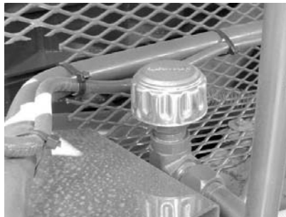
Figure 3-33 Oil tank (left), breather cap (center), ball valve (right)
