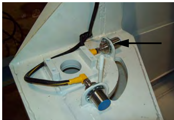
Figure 3-13 Packer blade ahead proximity switch
