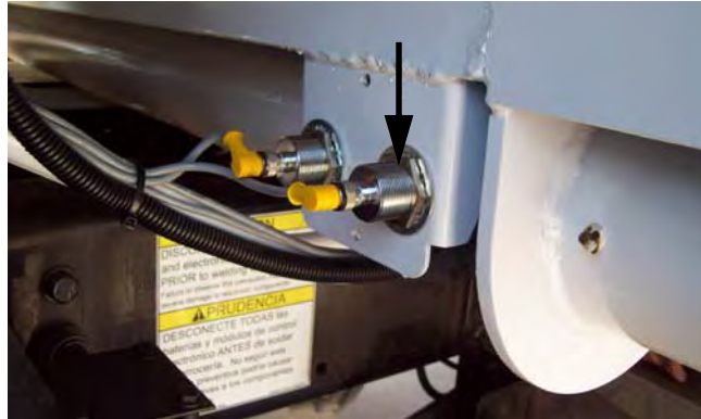
Figure 3-21 Arm fully retracted proximity switch
