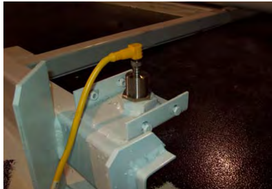
Figure 3-17 Tailgate fully open proximity switch
