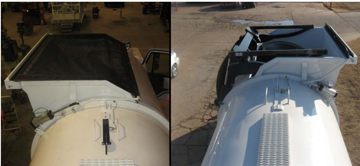
Figure 3-22 Closed tarp (left) / open tarp (right)
