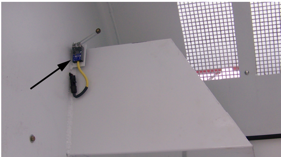
Figure 3-18 Fully retracted limit switch
