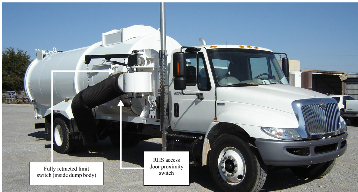
Figure 3-16 Switches on the curbside
