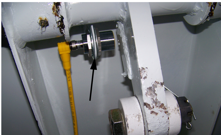
Figure 3-20 Tailgate locking proximity switch
