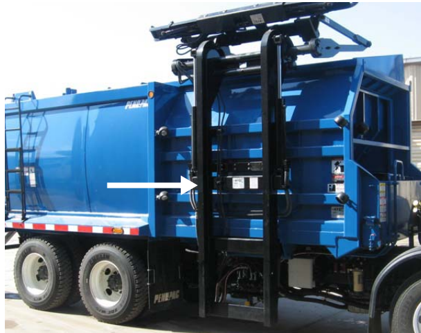
Figure 2-5 Slide retracted and in “HOME” position
