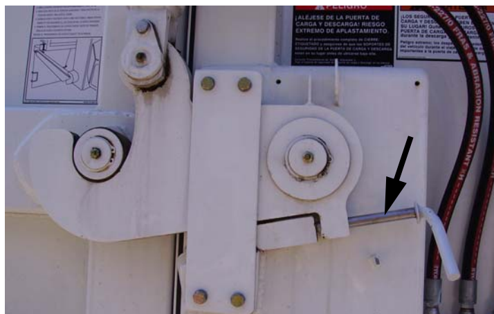
Figure 2-3 Tailgate safety lock in removed position
