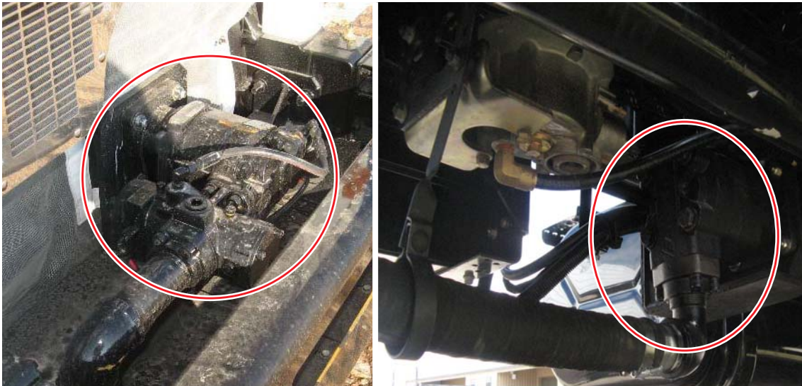
Figure 3-1 Front-mounted pump (left)/PTO-mounted pump (right)
