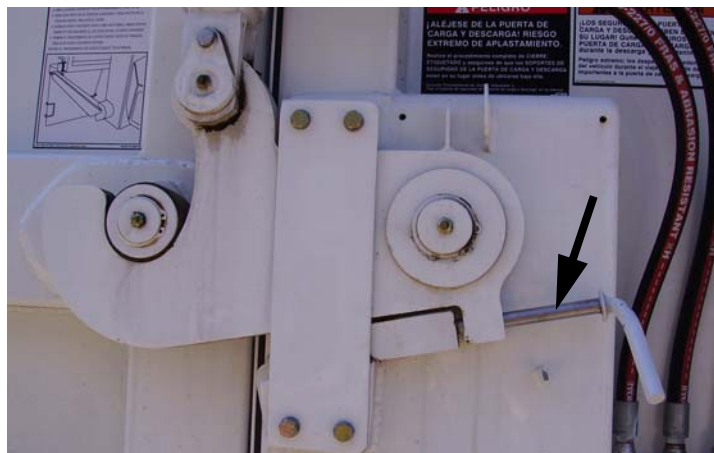
Figure 2-5 Tailgate safety lock in removed position
