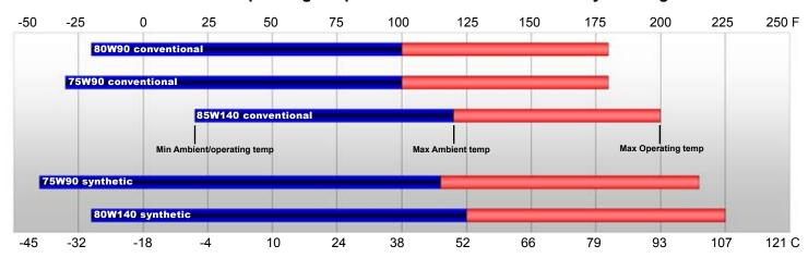
Note: Ambient temperature is the air temperature measured in the immediate vicinity of the gearbox. A gearbox exposed to the direct rays of the sun or other radiant heat sources will operate at higher temperatures and therefore must be given special consideration. The max operating temp must not be exceeded under any circumstances, regardless of ambient temperature.
