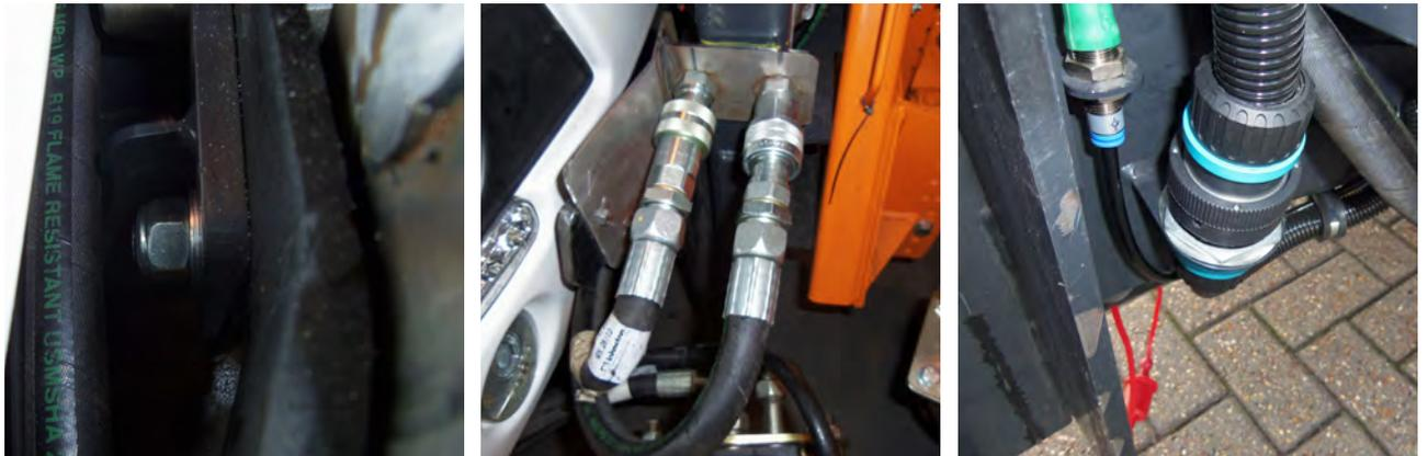
The snow plough/brush is now ready to fit onto the interface plate; utilising either mobile or static lifting equipment.
