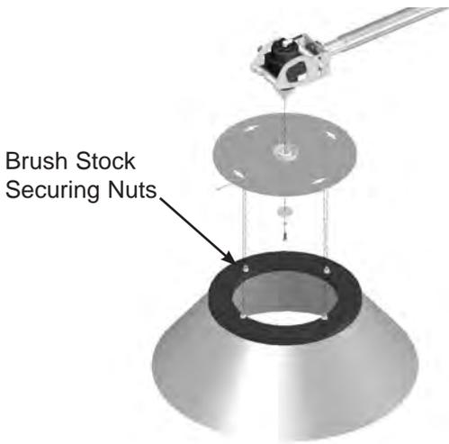
**Removal:** It is preferable to have the brushes in the working position and stationary. This is effected by stopping the engine with the sweep gear engaged. Release the four nuts from the bolts securing the brush stock to the driving plate, remove brush.
