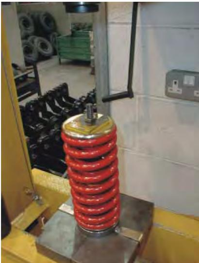
12. Once the damper top has been removed from the assembly, refit the special tool and spacer tube. Position the assembly on the press as before. Again, apply force to the special tool via the spacer tube until the fork plate from the special tool is loose. Remove the fork plate and carefully release the pressure of the press from the springs.
