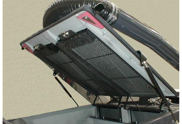
Refitting of the hopper mesh screens can be done either in the reverse order of removal, or it may be found easier to refit the meshes by fully lifting the hopper and offering up the mesh. The mesh should be lifted into the retaining channel and one at a time, the lynch pins should be fitted.
