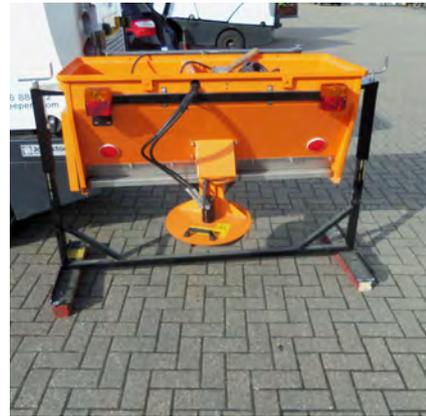
Once locating pins have been fitted the stand can be removed.
