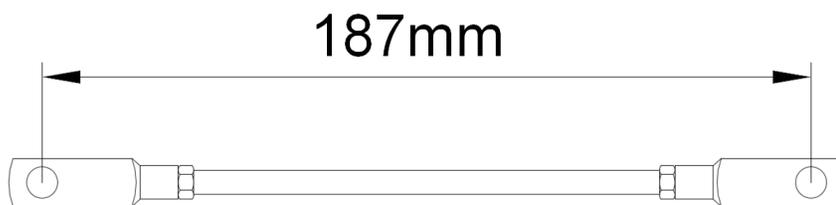
**Figure Three: Actuator Rod Length**
