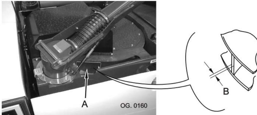
Remove plate (A) after releasing the two retaining bolts.
