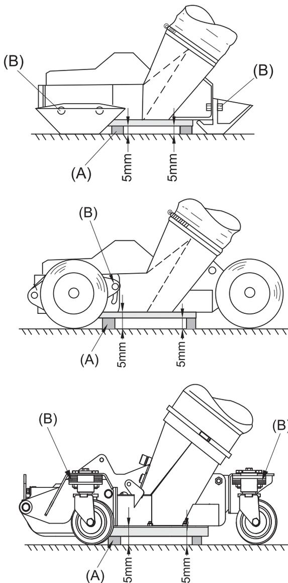
The adjustment is carried out by lowering the nozzle onto the 3 height setting anvils provided, then releasing the adjusting bolts and adjusting the nozzle to the desired height.
