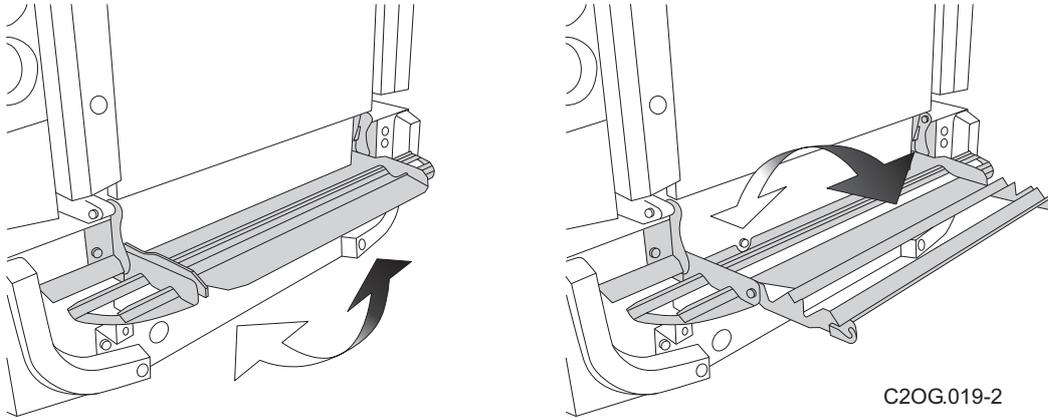
The step can be accessed by pulling the lower edge away from the machine and hinging it upward. It is secured by lifting it above a horizontal position and pushing it in towards the back of the machine and lowering it into the working position. There are location pins at either end of the grille. Ensure that both pins are engaged correctly. Open out the centre section.
