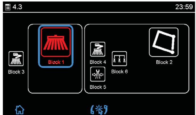
An example of a fault condition on a valve block is displayed opposite.
