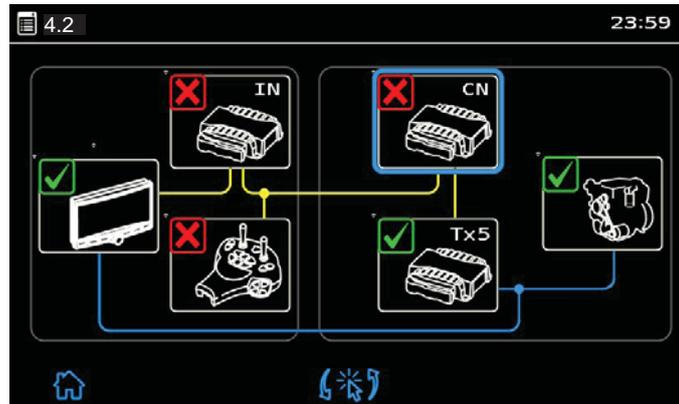
An example fault condition on the CANbus network is displayed opposite.
