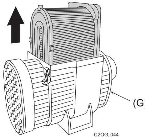
The safety element should be changed every third time the main element is serviced. Inspect the clean element for damage by placing a bright light inside and looking through the element. Any thin spots, pin holes or other damage will render the element unfit for further use.
