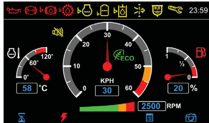
When work mode is selected (by selecting steering column switch H2b) the Work Mode Sreen will be displayed;
