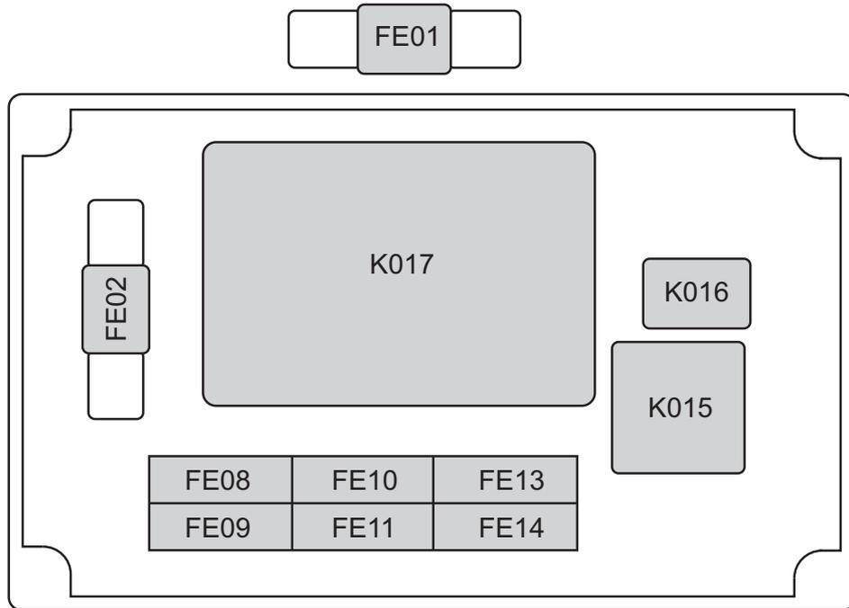
Access fuse by removing battery box cover.
