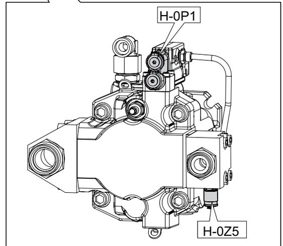
Test points are provided on the hydraulic system to carry out pressure checks.
