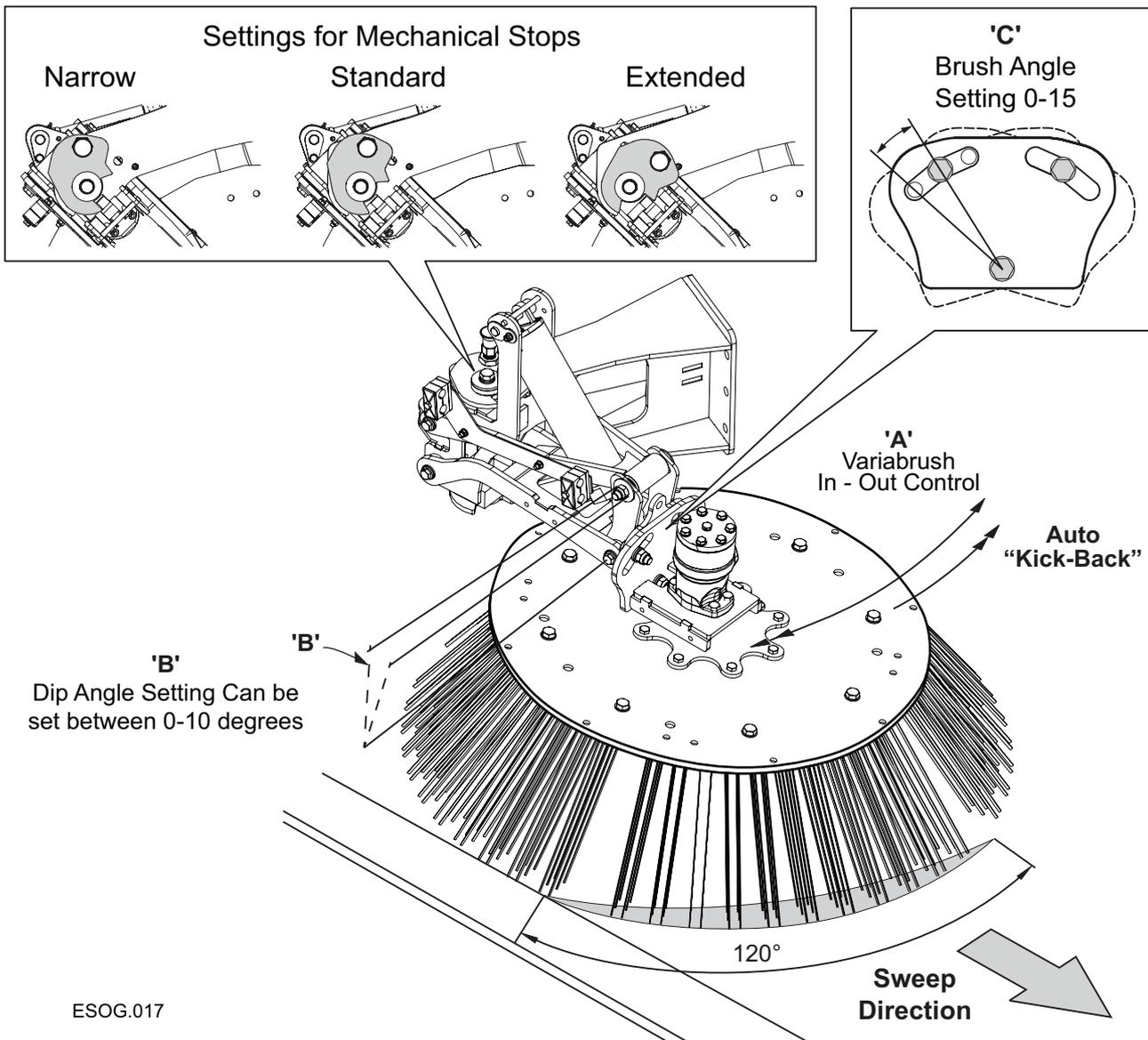
The brush angle should be set using adjustment (C) and (D) so that only about 120° of the circumference towards the front kerb is in contact with the road.
