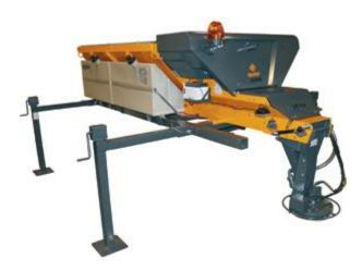
Like all other Epoke machines, IGLOO features surface treatment consisting of sandblasting, zinc dust priming, 2-component polyurethane base coat and a 2-component top coat. The spreading disc and feed funnel are made of stainless steel.
