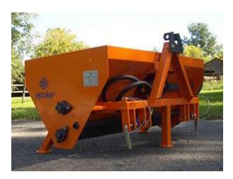
Driven by tractor hydraulics at a flow rate of 10 - 40 liters/minute[2.6 - 10.6 gal/min].
