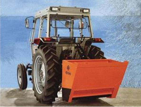
The PSL is built to be mounted on the tractor's three-point linkage and its construction as a loading bucket means that when the spreader is lowered, it can be filled by reversing directly into the spreading material. The tractor then pulls the spreader into the upright position and it is ready to work. It is hydraulically driven off the tractor's hydraulic system.
