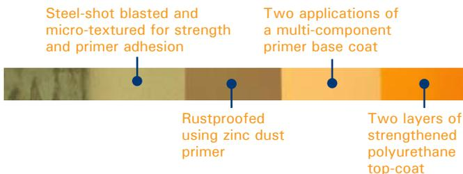
Combined with multi-stage curing treatments and stainless steel fasteners, this process provides optimum anti-corrosion protection, guaranteed for 10 years!
