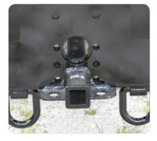
REESE RECEIVER / PINTLE HOOK Optional 2" receiver 3,000 lb. vertical load, 16,000 lb. gross trailer weight with LED light bumper. Pintle hook option comes with gladhands. The truck must have a trailer package at the rear (20k vertical and 100k tow rating)
