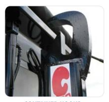
**CONTAINER HOOKS** Container jib hook meets DOT requirements for front container securement
