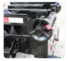
**REAR ROLLER** Optional rear rollers aid in loading and unloading the container
