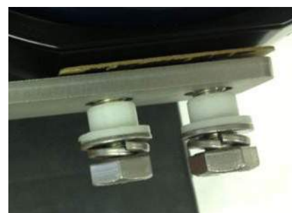
Illustration 19. Pump bracket mounting hardware assembly order. (Pre-tightening)
