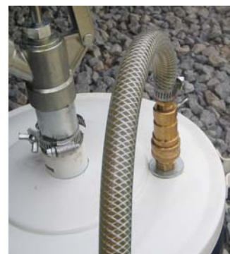
Illustration 36. Circulate grease to remove air pockets.
