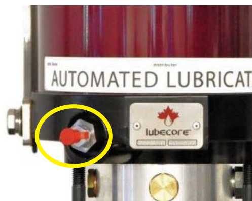
Illustration 37. Male filler coupling with dust cap. Either a regular grease zerk for EP2 grease or a male quick disconnect for EP0 grease.
