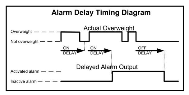
These delays are programmed in seconds, from 0 to 60. A delay of 0 means that the alarm output state reflects the overweight state, with no delay. This is the factory setting.
