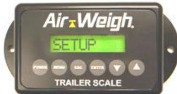
**INSTRUCT** - Select YES to include text reminders on the scale display during first start up. The reminders include weighing on a flat surface, releasing the brakes and inflating the suspension. Select NO to turn this feature off.
