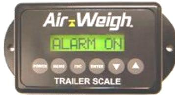
5. To activate the alarm feature, use arrows <▼ ▲> to display ALARM ON. Press <ENTER>. Choose YES or NO and then press <ENTER>. Scale momentarily displays *Accepted*.
