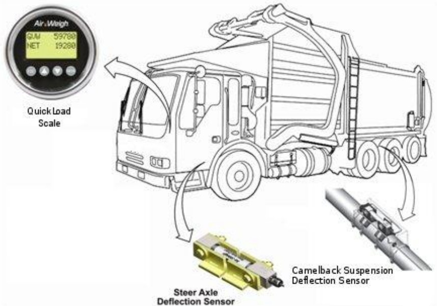
Figure 1. Major Components Location
