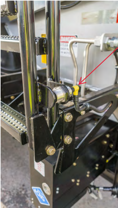
3. LADDER DOWN PROX SWITCH
