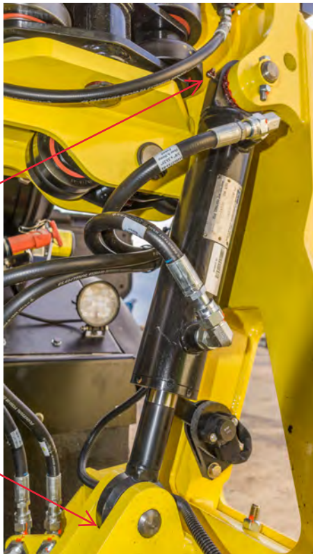
GRIP DRIVE LINKS [GREASE WEEKLY]
