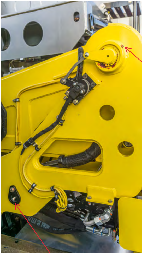
ARM LIFT CYLINDER BASE END [GREASE WEEKLY]
