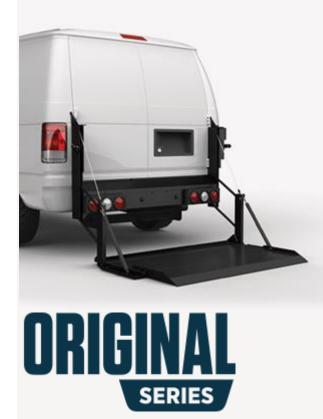
ORIGINAL SERIES Constructed with the same high-quality pumps and motors found in all other Tommy Gate lifts, Original Series liftgates use military aircraft-grade cable for added strength.
