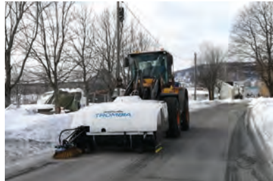
Sweeping in sub-zero temperatures. Trombia uses no water that can freeze the ground!
