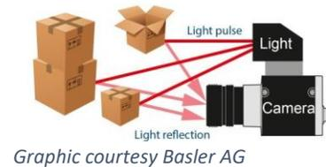
Because the TOF camera provides its own illumination source, its influence by ambient light is low, except where IR may be present, as in sunlight. TOF cameras are also relatively compact with a fast scan rate. Disadvantages are lower resolution and higher cost than some 3D options.
