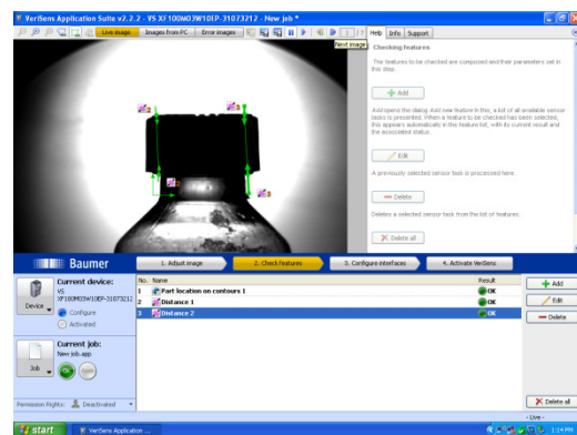
FIGURE 2: GOOD PART SHOWN WITH INSPECTION TOOLS
