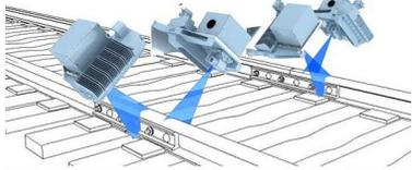
In these systems the light sources and cameras are often mounted to the bed of a truck equipped with rail wheels. As the truck drives along the rails, images are captured and stitched together and analyzed with sophisticated software. These systems automatically inspect of rail joints and rail sides for cracks, missing bolts, corrosion, welds and electrical connections. As with AUVIS, these systems must be very rugged and able to withstand temperature and moisture extremes.
