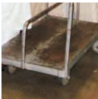
Metal—dents and rusts
