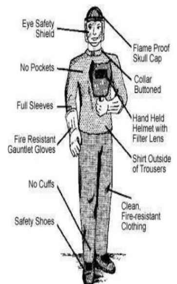
Figure 1 PROPER PROCEDURE FOR WELDING IN A TANK
