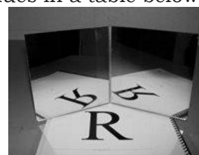
Figure 8. Multiple Images Formed by Two Plane Mirrors at 90^\circ Angle
