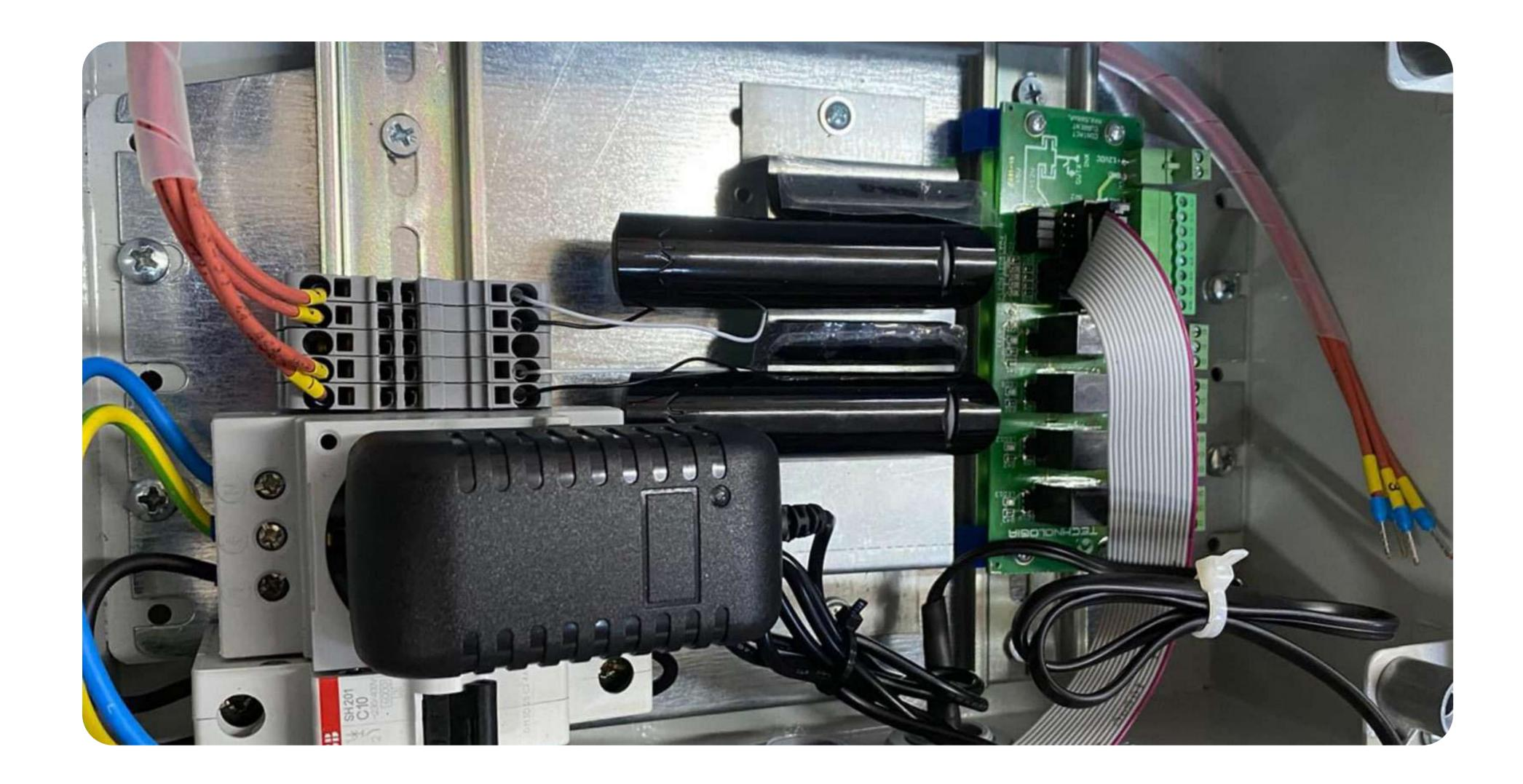
In its turn, the WallSwitch power relay is connected to the mains of the ventilation, irrigation, heating, and air cooling systems.
