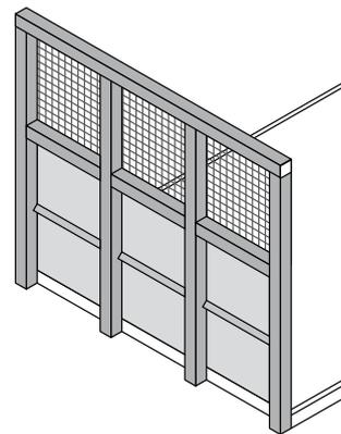
*Figure 365 Reinforced "pipe gate" style load rack*
