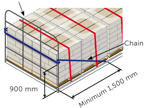
*Figure 373 Chains should be kept below 30°*
