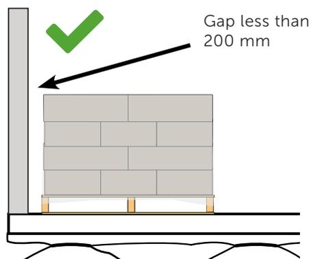
*Figure 370 Unblocked load*
