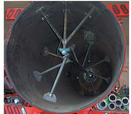
A common "Mechanical Paddle" style agitator in a vac truck tank
