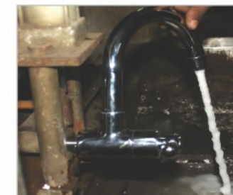
FINAL TESTING OF EVERY PRODUCT ON HYDRAULIC PUMP BEFORE PACKING
