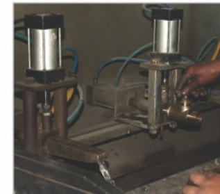
TESTING OF FLOW & LEAKAGE OF EACH AND EVERY PRODUCT AFTER MACHINING ON HYDRAULIC TESTING PUMP
