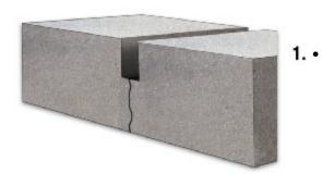
Clean out Joint with diamond blade to provide a clean porous surface.
