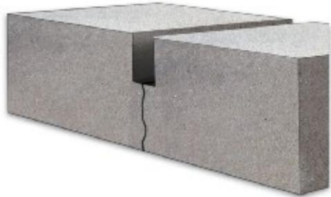
1. • Clean out Joint with diamond blade to provide a clean porous surface.
