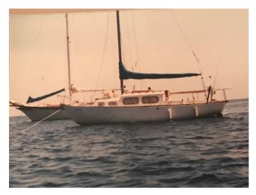
After our return to Dana Point, we started looking for a little bigger boat. We got a 26-foot Columbia sailboat. It had an 8-foot beam, 4-foot draft, 2300 lbs. Lead Ballast, 5200 lbs. displacement, 25-gallon water tank, 6 feet standing head room, full main and jib. We started preparing and outfitting the boat for our next cruise.
