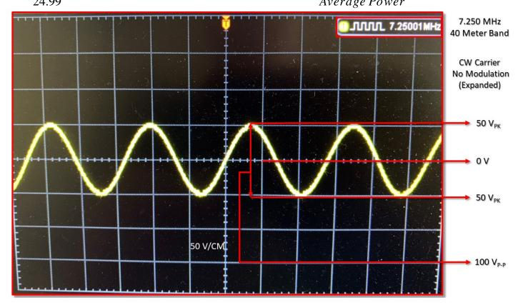
This photo is identical to the one above, except in this one, the oscilloscope trace has been expanded out to show the actual sine wave of the carrier frequency as noted by the frequency counter readout in the upper right hand corner. It is still a continuous wave.
