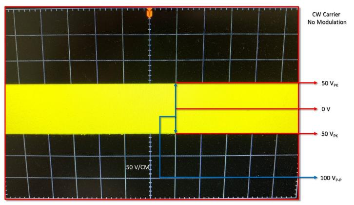
This photo illustrates the same carrier wave without any modulation. It's just 7,250,000 Hz. sitting there all by itself. This is what we call Continuous Wave (CW). If we were to transmit this signal on an HF transmitter, and then tune a receiver away from 7.250 MHz., let's say to about 7,250,500 Hz., we would hear a steady tone.
