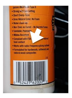
For some electronic projects, **Gorilla Wood Glue** can be used for RF applications. I have used it to secure windings on coils.
