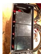
volt, 7 amp sealed lead acid batteries inside a Harbor Freight ammo **box** wired in parallel giving me 12 volts, 21 amps. The ammo box was on sale
