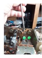
A tiny drop of grease on the tip of a Phillips screwdriver will hold a screw to the screwdriver in order to reach down into a space too small to
