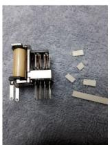
Use thin strips cut from a brown paper bag or the strips cut from unprinted portion of textured white business cards to clean relay contacts. This method will clean and burnish contacts without removing any contact plating. Snip off the dirty tip of the strip and continue burnishing until the paper comes through the contacts clean. (Arnie, KD6CZ)
