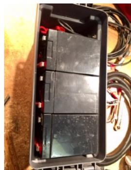
volt, 7 amp sealed lead acid batteries inside a [Harbor Freight ammo box](#) wired in parallel giving me 12 volts, 21 amps. The ammo box was on sale
