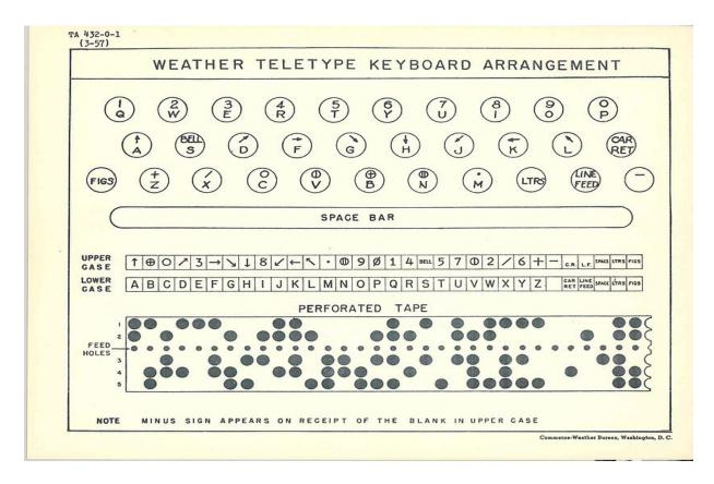
Let's take this concept apart a little bit. We'll look at the second form of digital communications, the first being CW (Morse Code). The second form of digital communication is Radioteletype (RTTY). RTTY utilizes the Baudot Code.
