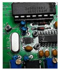
Figure 6: Carefully align the new IC and solder in place with very tiny amount of solder. Verify all pins are soldered with no solder bridges. A jeweler's Loupe comes in very handy
