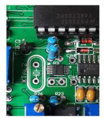
Figure 2: First some surrounding components were removed to give better access to the IC.
