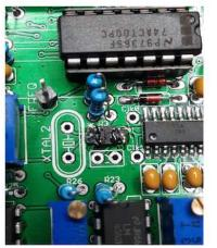
Figure 3: melt a blob of SMD Removal Alloy to cover all of the IC pins.
