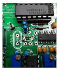
Figure 4: Reheat the Alloy (it stays molten for several seconds) and remove IC with tweezers.
