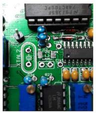
Figure 5: Clean the Removal Alloy from the board using fluxed solder wick.
