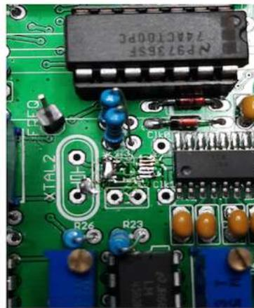
Figure 4: Reheat the Alloy (it stays molten for several seconds) and remove IC with tweezers.
