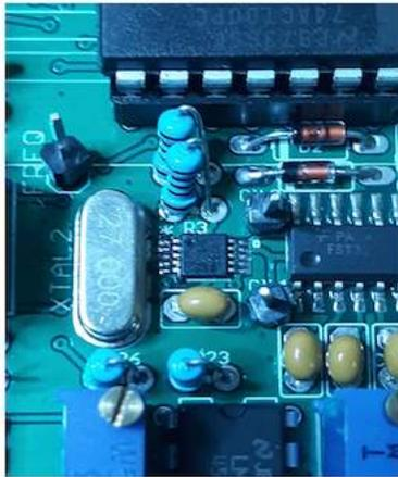
Figure 1: The Chip to be replaced is located just to the right of the 27.000MHz crystal
