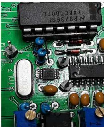
Figure 6: Carefully align the new IC and solder in place with very tiny amount of solder. Verify all pins are soldered with no solder bridges. A jeweler's Loupe comes in very handy
