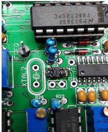
Figure 3: melt a blob of SMD Removal Alloy to cover all of the IC pins.
