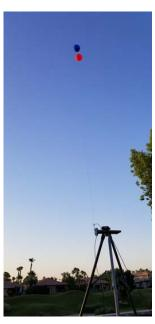
The antenna was adjusted in length to be halfwave at both 40m (64.8') and 80m (123.2').The slight breeze converted the vertical to a sloper which was OK. The only major
