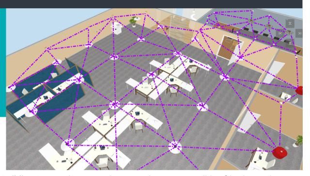
For a **Total Building Automation** network you need a system capible of having each device talk directly to any other device within its range and also be able to communicate with devices anywhere across the entire building or campus. This nessesitates the use of a massive mesh network structure.
