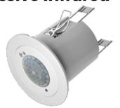
PIR sensors that detect only human movement are used to trigger lighting in common areas and switch off lighting when spaces are empty. These same sensors also detect the amount of daylight coming through windows and skylights.
