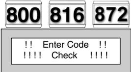
In the event of a Mains Power Failure the display will show:-
